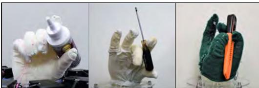
Figure 7.7.: Demonstration of static grasping with a glue bottle (left), a screwdriver (middle) and a box cutter (right).
