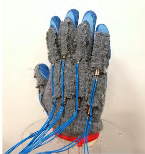
Figure 7.2.: Custom sensor glove on a foam robot hand.
