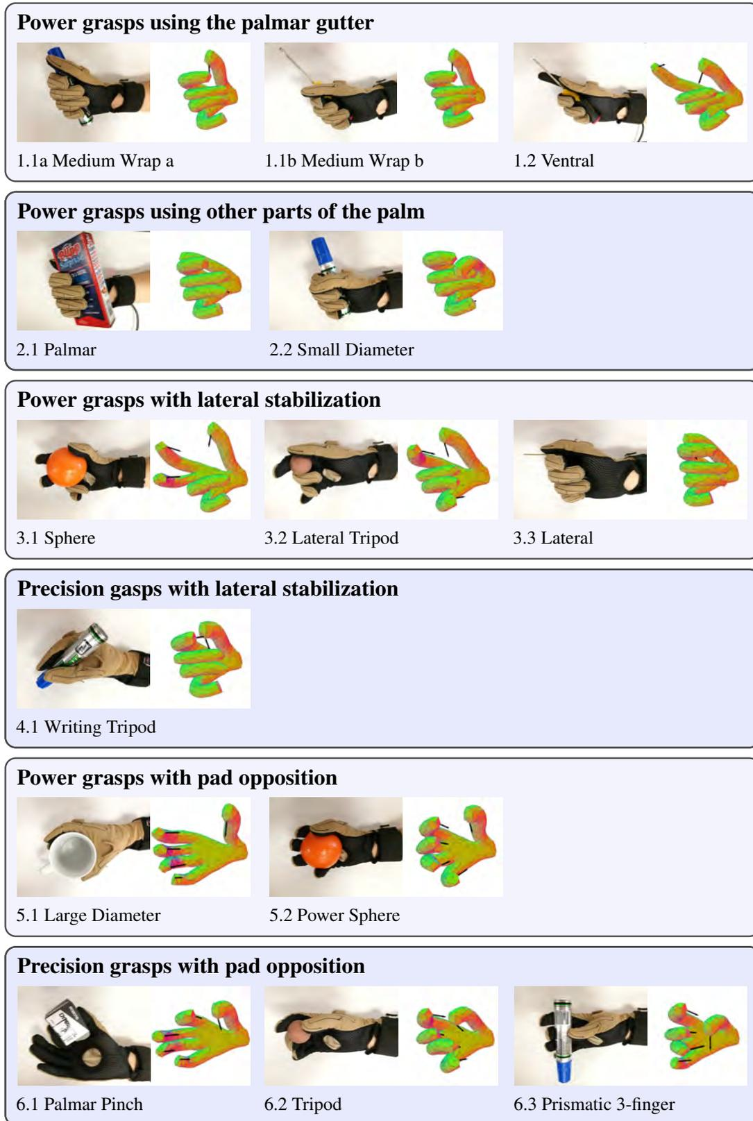
Figure 6.10.: 14 Target grasps recorded with a CyberGlove, transferred to simulation poses. For each grasp, the left image shows the target grasp, and on the right, the configuration of the deformed simulation mesh is shown, including surface normals (black arrows) of fingertips. *Image by Dominik Bauer.*
