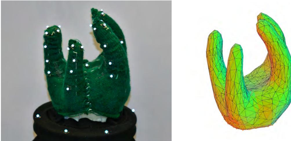
Figure 6.5.: Left) Four finger hand with markers. Right) Simulation mesh of the same hand model. The simulation mesh is anchored in the world coordinate system by pins on the bottom nodes of the mesh.
