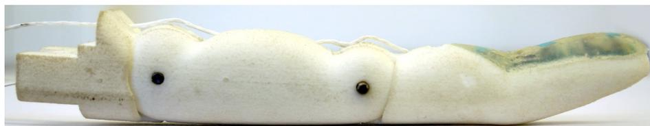
**Figure 4.** Profile of the ring finger showing a curved design for the individual phalanges
