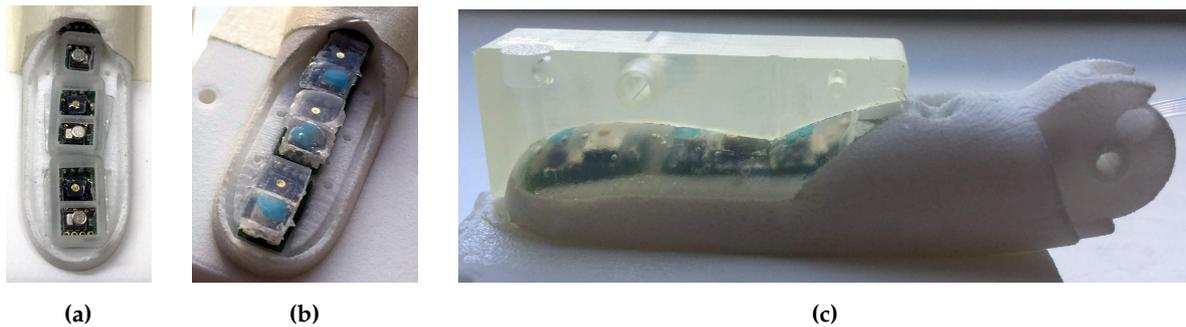
**Figure 7.** (a) The moulds for the silicone rubber casting process are placed directly into the finger. (b) The individual sensors have been cast in rubber. The next step is to cast the remaining finger pad area in rubber. (c) The result of the casting process of the finger tip and one half of the used mould is shown. A silicone canal is used to inject silicone rubber into the moulds.
