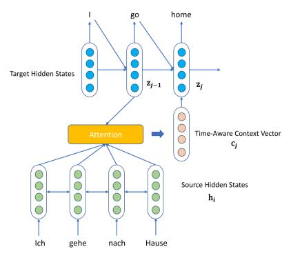
FIGURE 3.4: Recurrent NMT architecture with attention.
