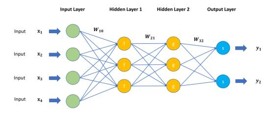
FIGURE 2.7: A multi-layer perceptron with three layers.
