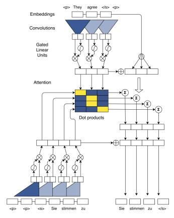
FIGURE 3.5: Convolutional NMT architecture (Gehring et al., 2017).
