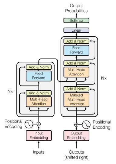
FIGURE 3.7: Transformer Architecture for NMT (Vaswani et al., 2017).
