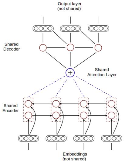
FIGURE 5.3: NMT architecture with shared components.
