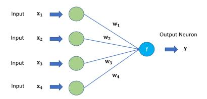
FIGURE 2.5: Linear models with a single output neuron.
