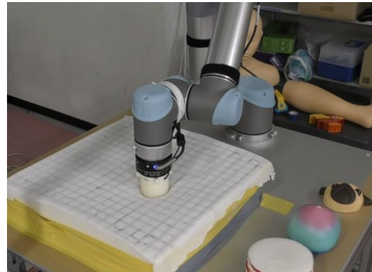
Fig. 5.12.: UR5 probing foam material to generate reference deformation data
