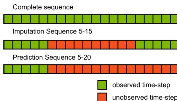
Fig. 5.5.: Imputation [5-15] and prediction [5-20] schematic illustration
