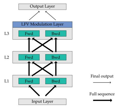
**Figure 4.3:** BiLSTM network architecture. The full sequence gets propagated through all BiLSTM layers. At the last layer, only the final output is retained, being modulated and forwarded to the output layer.
