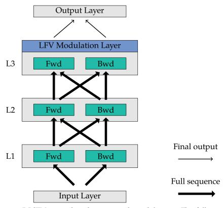
**Figure 4.9:** BiLSTM network architecture with modulation. The full sequence is propagated through the BiLSTM layers. Only the final output is retained after the final BiLSTM layer, being modulated and forwarded to the output layer.
