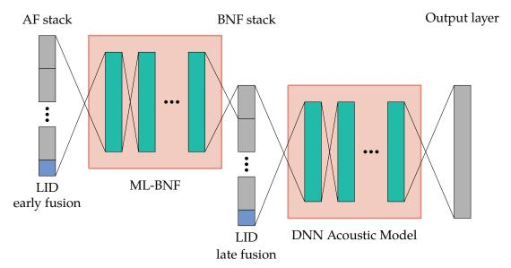
**Figure 6.2:** Overview of the network architecture used in our setup. We first stack the acoustic features (AF) and append a language identification (LID) code, before feeding them into the ML-BNF network. The ML-BNFs are stacked as well and the LID code is again added. The second DNN computes the phone posteriors as part of the acoustic model.
