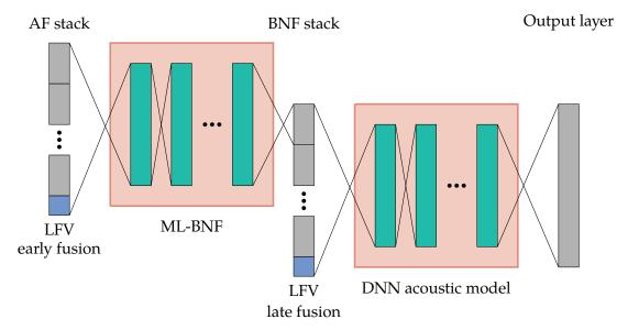
**Figure 6.7:** Overview of the network architecture used in our setup. We first stack the acoustic features (AF) and augment them with language feature vectors (LFV) before feeding them into the ML-BNF network in order to extract adapted ML-BNFs. The ML-BNFs are stacked as well and the LFV code is added again. The second DNN computes the phoneme posteriors.
