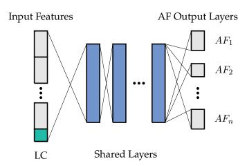
**Figure 4.2:** Network architecture of DNN based articulatory feature detectors using multi-task learning (MTL): the hidden layers were shared, while individual output layers for each articulatory feature were used. Language codes (LC) were optionally supplied.
