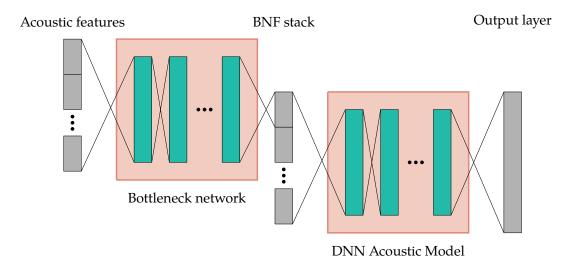
**Figure 2.4:** Overview of the network architecture used in hybrid DNN/HMM systems. Starting with the stack of the acoustic features, BNFs are extracted, stacked and used as input to the DNN acoustic model, which computes the phone posterior probabilities.
