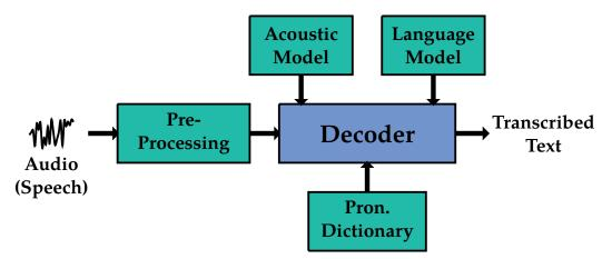
Figure 2.1: Components of an ASR system.
