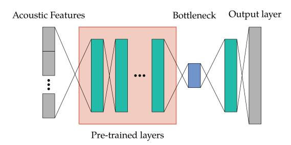
Figure 2.3: Network for bottleneck feature (BNF) extraction.
