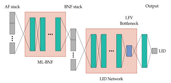
**Figure 6.3:** Overview of the network architecture used for LFV extraction. We first stack the acoustic features (AF) as input to the ML-BNF in order to extract BNFs. The BNFs are stacked and input into the LID network. This DNN is trained for language identification.
