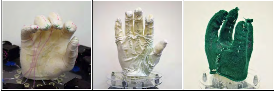
Figure 3.1.: Soft foam hand robot prototypes. Left : Initial prototype, anthropomorphic hand in a 'cupped' rest pose. Middle : Anthropomorphic hand in a stretched out rest pose. Tendons only run on the inner side of the hand. Right : Non-anthropomorphic four fingered gripper.
