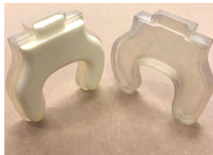
Figure 3.5.: 3D printed mold and foam cast for a 2D planar gripper foam robot.
