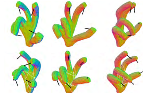
Figure A.1.: Optimization results for the 14 selected grasps (1). Top: Target pose. Bottom: Resulting pose.
